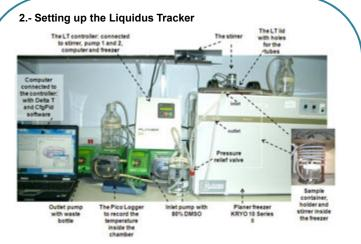
Alginate encapsulated liver cells are added to the sample container which is placed inside the controlled rate freezer of the Planer Liquidus Tracker. The CPA concentration of the sample is increased by pumping a highly concentrated CPA solution into the container while the freezer cools down. A stirring system mixes the CPA concentration to achieve a homogeneous concentration (developed by Planer and David Pegg).
